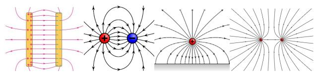
The diagrams above show the electric field lines around positive and negative point charges. Field lines generally point from **positive to negative**, are **equally spaced** as they exit a surface and are **perpendicular to the surface**. Lines that stretch from a positive charge to a negative charge show attraction whereas field lines that do not join up identify repulsion. Here are some other common geometries.
