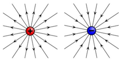
Protons and electrons are charged particles that can be modelled as **point charges** i.e. their charge exists at a single point in space. Point charges have **radial fields** which look like the spokes of a wheel. Electric field lines point outwards from a positive charge or inwards towards a negative charge as the direction of the field represents the direction of the electrostatic force on a positive charge at that point. The strength of the field decreases with
