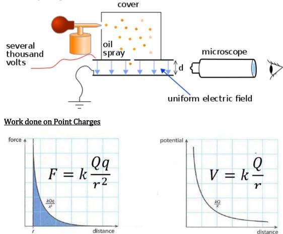
Work is done when a charge, q, is brought in from infinity to a distance r from a point charge, Q. This work is the electrical energy of this geometry. The graph on the left shows the force needed as a function of the distance between the particle and the point charge. The work is the area underneath this graph from infinite separation to the distance between the charges, r.
